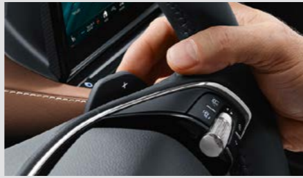
2-spoke leather heated multi-function steering wheel with paddles for recuperation level selection
